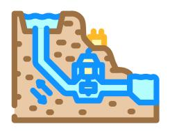
Pumped hydro uses two reservoirs at different heights and moves water between these reservoirs. During times when electricity is needed, water moves from the higher reservoir through a turbine generator to the lower reservoir. During times when electricity is not needed, an electric motor pumps water from the lower reservoir to the higher reservoir.
